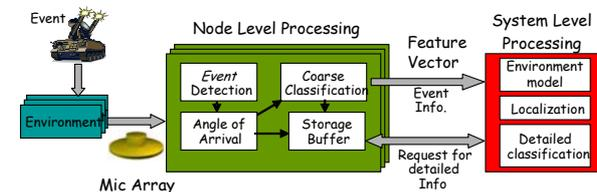
Figure 1: Networked acoustic array and tracking system.
