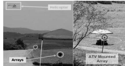
Figure 3. Experimental Setup to Track helicopter.
