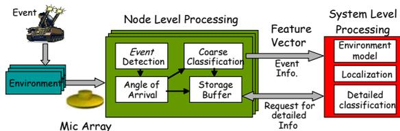
Figure 1: Networked acoustic array and tracking system.
