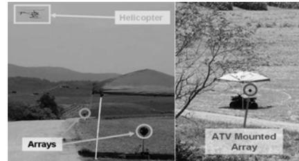
Figure 3. Experimental Setup to Track helicopter.
