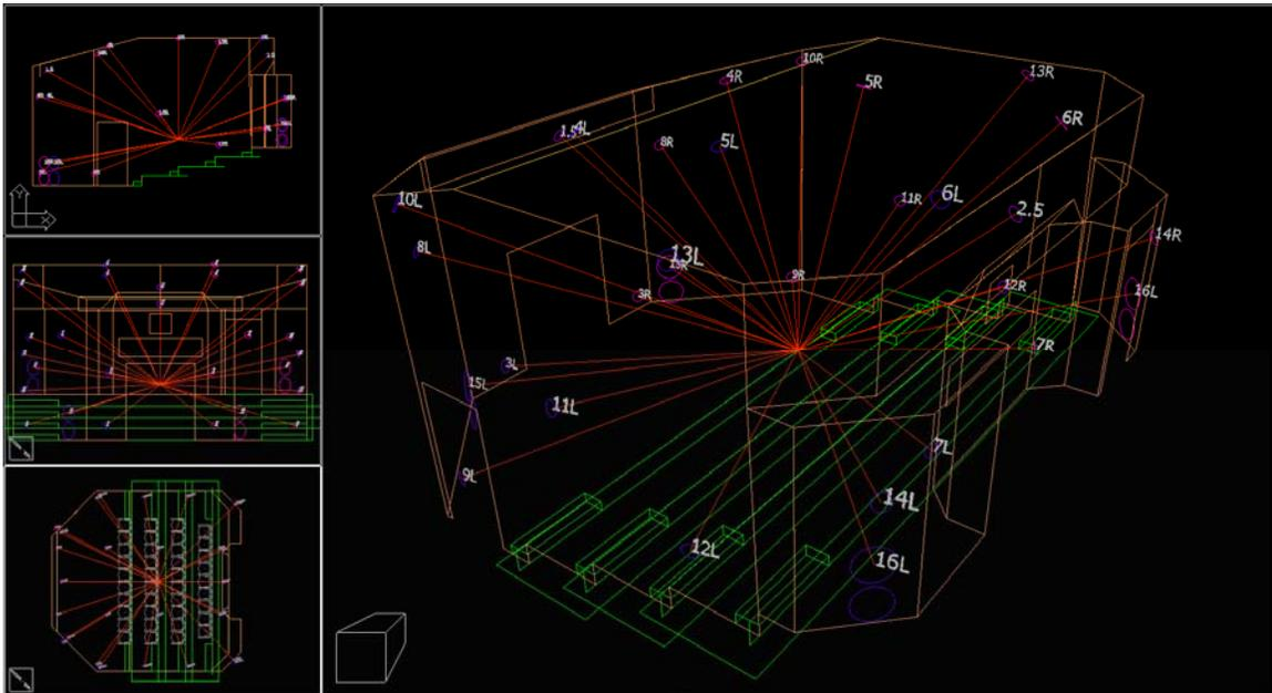
**Figure 1 – VBAP 32-loudspeaker arrangement for an auditorium.**
