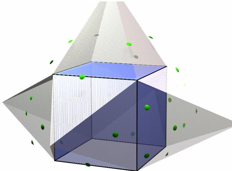
Figure 3 – VBAP 32-loudspeaker arrangement for a six-sided CAVE.
