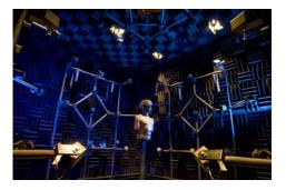
The room contains 57 test loudspeakers separated by 30 degrees in vertical and horizontal directions and constituting a sphere surrounding the listener.
