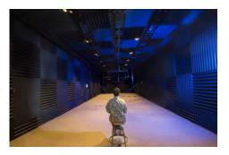
The main sound projection system of the Distance Hall consists of 180 loudspeakers arranged in linear groups of five that are suspended from the ceiling every 5 feet along the length of the hall in three parallel lanes to form 12 rows of 15 loudspeakers each across the hall.
