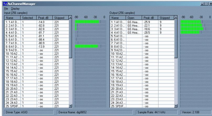
Under normal operation, the GoldServ application will launch the ChannelManager automatically when needed. By default, metering within the ChannelManager is disabled. To enable ChannelManager metering, choose Display->Meters from the menu.
