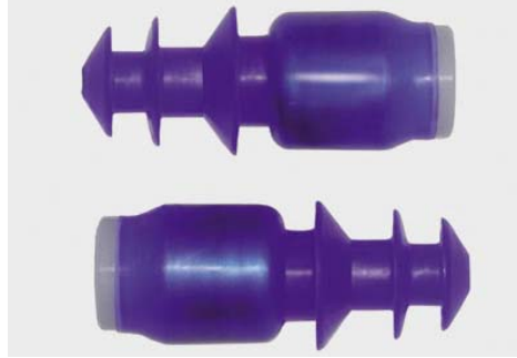
Figure 3: Silencio Super-Sound Bafflers FUN-85 are a good example of a flanged, passively activated in-ear hearing protector. Normal sound pressure levels are passed through its orifice, while a diaphragm is forced closed by high-intensity sound pressures.
