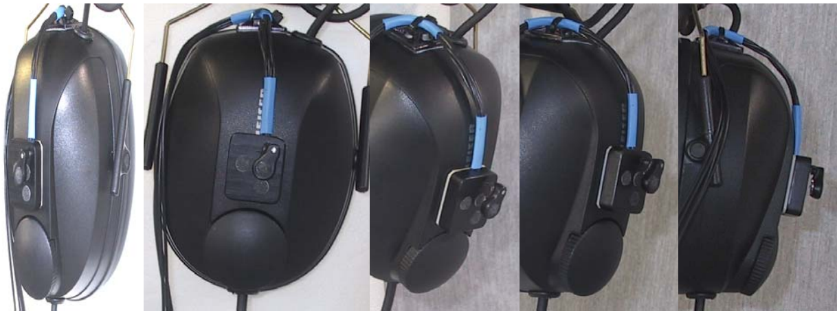
Figure 42: Compact sound-field microphone as mounted on Sennheiser HD205 muff. The array may be covered/protected with a hardwire cage and foam windscreen. The location is centered over the ear canal with respect to the sagittal plane, and thus on the interaural axis.
