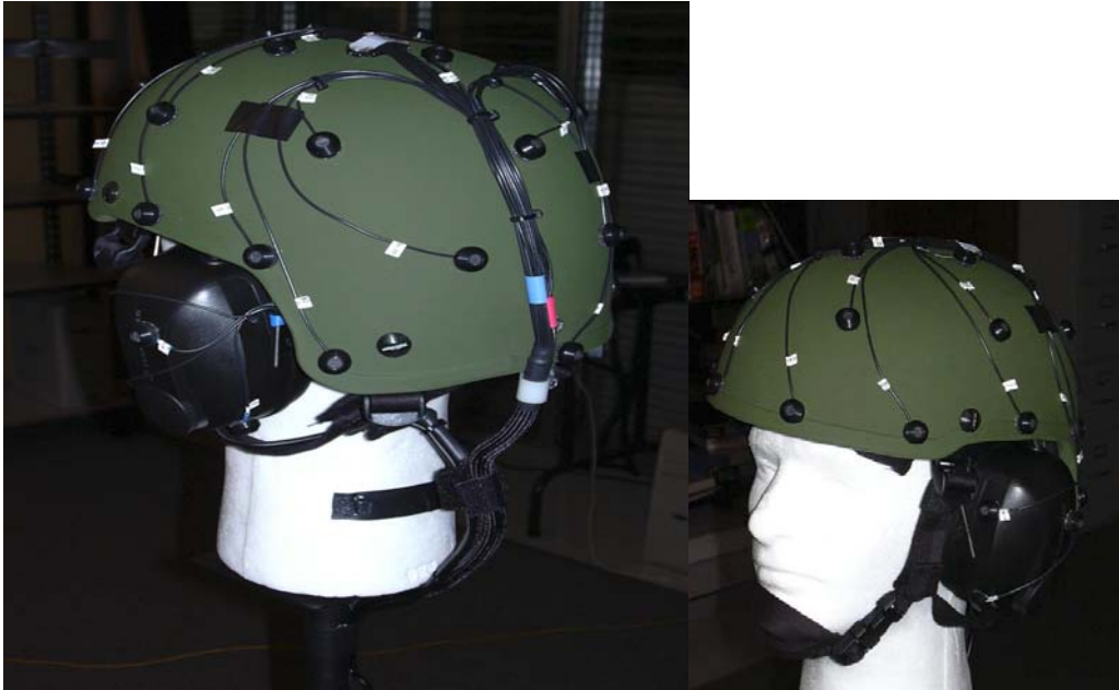
Figure 30: 32-channel system prototype, showing 4 microphones located on each muff, 4 microphones on the sagittal plane of the helmet, and 10 pairs of microphones reflected on each side of the helmet.
