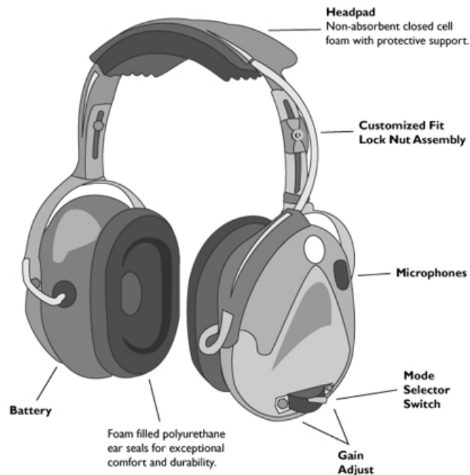
Figure 6: Gentex's Wolf Ears are a stereo Transparent Hearing System specifically designed for hunters. This system has four main settings: passive hearing protective device only (with a protection of 26 dB), a hear-thru hearing protection device (limiting all sounds to 84 dB SPL), transmission of all sounds at a constant level (automatic gain), and 6 dB amplification boost of all sounds (limited to 90 dB). The left and right speaker channels can be adjusted independently.
