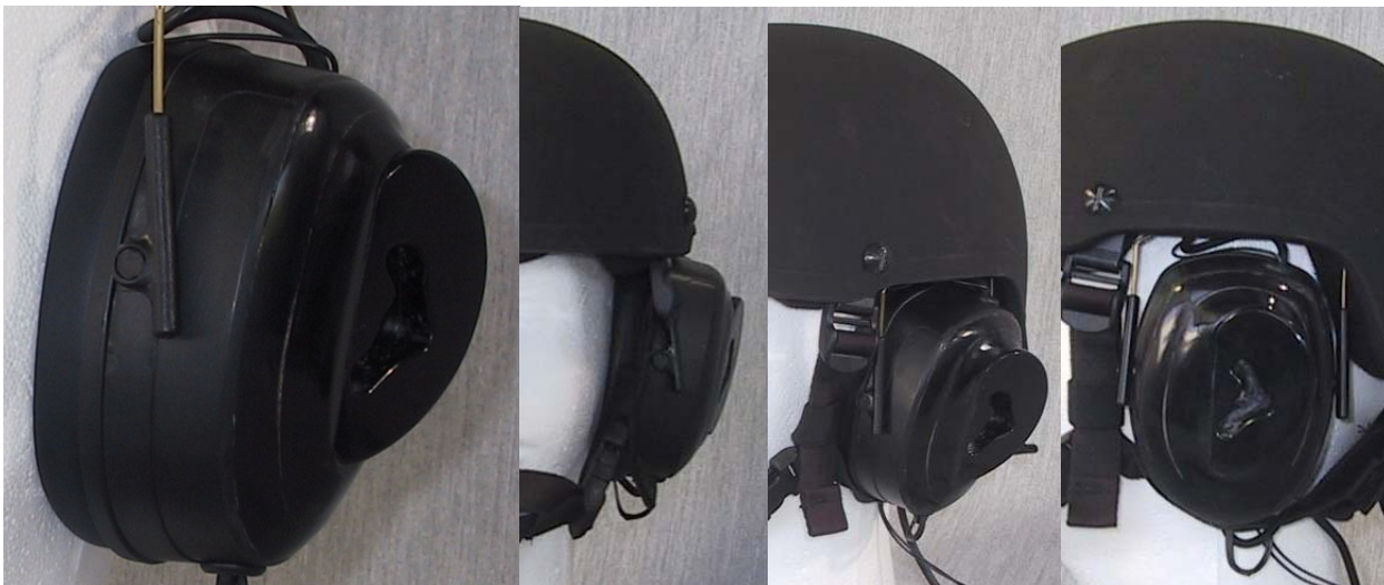
Figure 38: Hard Pinna mounted on muff for mechanically modeled pinna approach. The concha has human-replica features. The outer pinna is a much simplified baffle compared to a human equivalent. The ear canal depth is approximately 8 mm.
