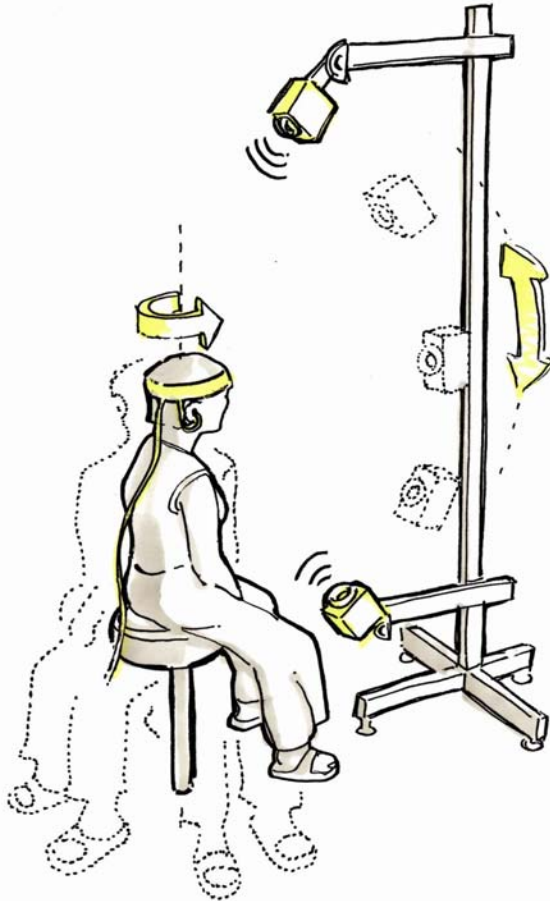
Figure 78: HeadZap apparatus operation, showing the two degrees of freedom: 1) one or more loud-speaker positioned along an arc, and 2) the subject turning to a select number of bearings.
