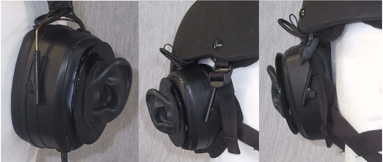
Figure 35: Multiple-views of the muff-mounted human-replica pinna system. The extra flange just outside the outer edge of the muff is the constraining ring for the optional windscreen, not shown.
