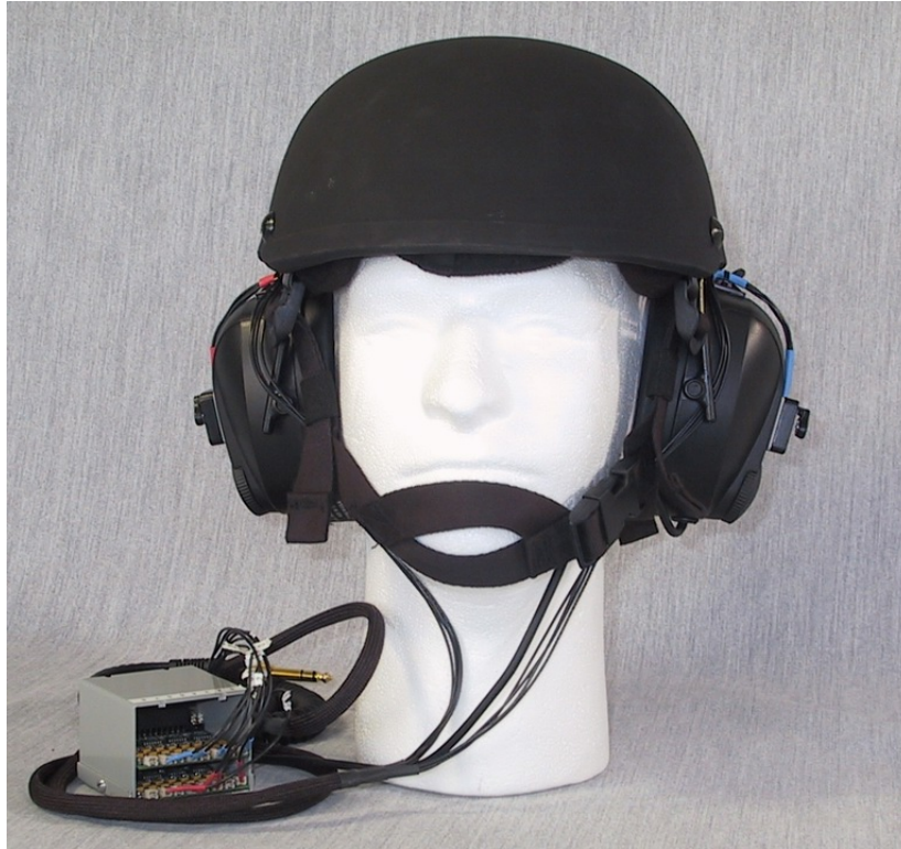
Figure 40: Helmet-integrated sound-field microphone approach. The sound-field microphone on each muff is a geometrically constrained array of 4 electret capsules. To support a total of 8 mic capsules, an 8-channel pre-amplifier is employed to interface the device to a digital processing.
