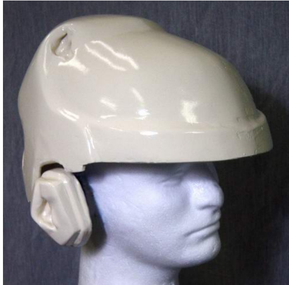
Figure 39: Human-modelled concha integrated into a helmet system. In this case, a concha replica was integrated into alternative positions: on the muff and on the helmet at an approximately correct interaural distance.
