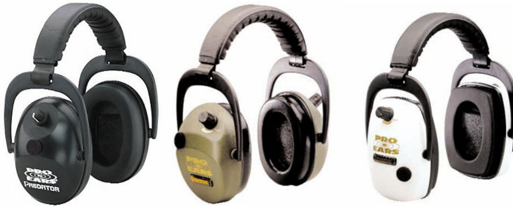
Figure 5: RidgeLine's ProEars are a stereo Transparent Hearing System with two microphones mounted flat against the earmuff. The left and right channels have independent manual and automatic volume controls. Loud sounds are attenuated to 70dB with an attenuation attack time of less than 2 msec, while all sounds below 70dB may be amplified up to 70dB.
