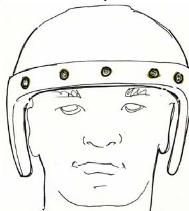
Figure 55: MicPlacement_3 Radial mic array naturally located along existing R2 channel
