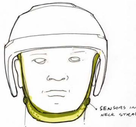
Figure 53: MicPlacement_2 Mics located on neck strap to align with inter-aural distance and provide ground sensitivity
