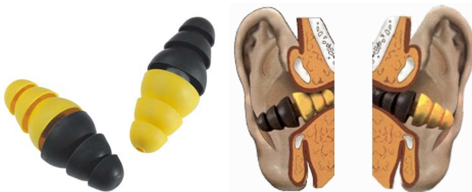
Figure 4: The Combat Arms Earplug is a dual-use device, where one orientation (brown in the ear canal) is a total plug and other (yellow in the ear canal) is a passively activated hear-through protector.
