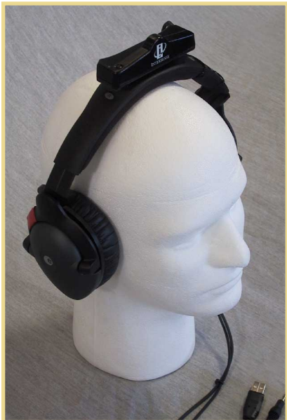
Standard Sennheiser eH2200 headphones, with mounted InterSense InterTrax2 tracker.
